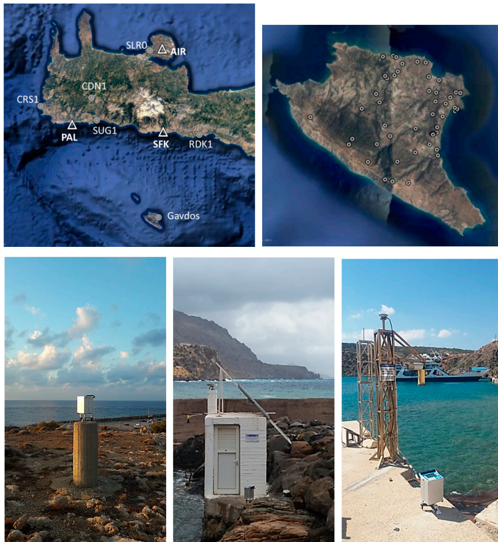
Figure 9. Terrestrial gravity measurements carried out in 2018 at various locations around the PFAC Cal/Val sites in Crete (top-left) and Gavdos (top-right). Locations with known absolute gravity values are marked with a triangle. Gravity observations are shown at the PAL absolute gravity point in south Crete (bottom-left), the RDK1 (bottom-middle) and Karave/Gavdos (bottom-right) Cal/Val sites.
