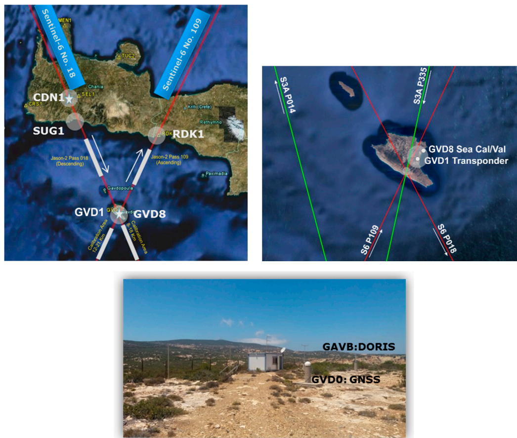
Figure 30. The location of the GVD1 transponder Cal/Val site in Gavdos island is under a crossover of the Sentinel-6 descending Pass No. 18, its ascending Pass No. 109 and the descending pass of Sentinel-3A Pass No. 335. The land of GVD1 is property of the Technical University of Crete. A permanent GNSS station has been operating there since 2004 (GVD0) whereas a Doppler Orbitography and Radiopositioning Integrated by Satellite (DORIS) beacon (GAVB) also operated for almost a decade (start 27-September-2003, end 27-March-2014).
